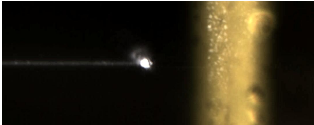
(b) The microsphere in contact with the surface, on top of the waveguide.
